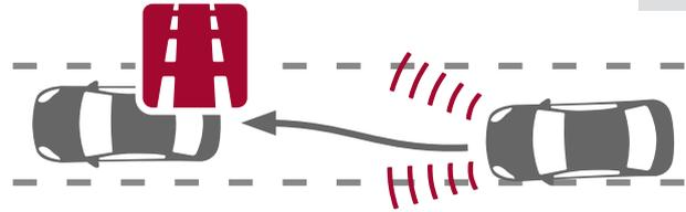
The **lane-keeping system** detects road markings on the right and left side of the vehicle with its sensors and determines the position of the vehicle in its lane. If the vehicle approaches the limits of the lane, or crosses them without turning on the indicator, the driver is first warned visually, and then acoustically or haptically. If the driver continues to approach the limits of the lane despite the warning, the vehicle is placed in the centre of the lane by braking or steering.
