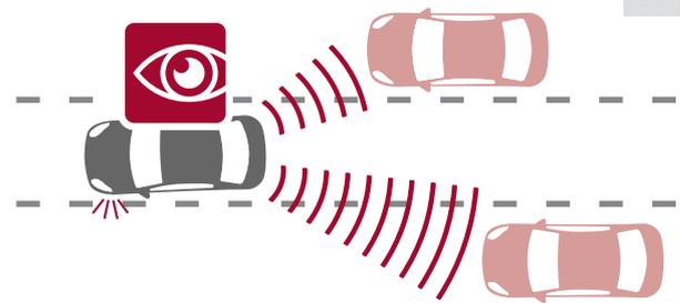
The **lane change assistant**, which was introduced in **2011**, monitors the areas on the sides and behind the vehicle (the so-called blind spots), recognizes vehicles in these areas, and informs the driver in a suitable manner. If the driver initiates a lane change although there is a vehicle in the monitored area, the driver is visually and/or acoustically warned by the lane change assistant.
