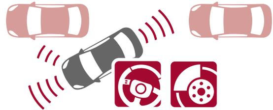
Parking and manoeuvring assistant with these specifications will be offered for the first time in new vehicles in **2017**. Regarding the previously known and widespread parking assistants with optical and/or acoustic warning, no damage-reducing effect could be detected.<sup>12</sup>
