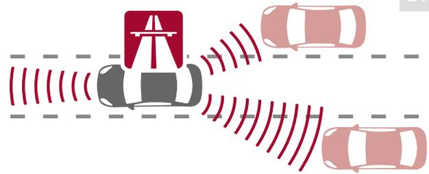
The **motorway pilot** is an automated driving system for motorways or motorway-like roads. Due to restrictions on such roads, control of cross traffic is not required. The first motorway pilot, which is initially designed up to a speed of 60 km/h only, will be introduced in **2017**. The driving task is returned back to the driver with sufficient lead time, for example, before leaving the motorway or near road works.
