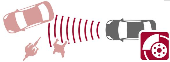
The **Emergency braking assistant** detects moving and stationary vehicles ahead, warns the driver in good time before an imminent collision and, if necessary, initiates partial or full braking to prevent the imminent collision. No limitation of the speed range is assumed. For the first time, emergency braking assistant was offered in new vehicles in 2013.
